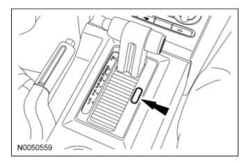
3. Using a suitable tool, press the brake shift interlock override mechanism on the transmission selector lever assembly, apply the brake pedal, press the button on the transmission selector lever knob and move the transmission selector lever into NEUTRAL.
